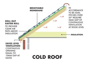
On a cold roof, insulation is placed between the floor joists meaning that there is little to no loss in height - although space for ventilation is required. It is called 'Cold Roof,' not because it is cold as such, but because it is slightly less efficient than a warm roof, this is because the rafters themselves remain uninsulated.
